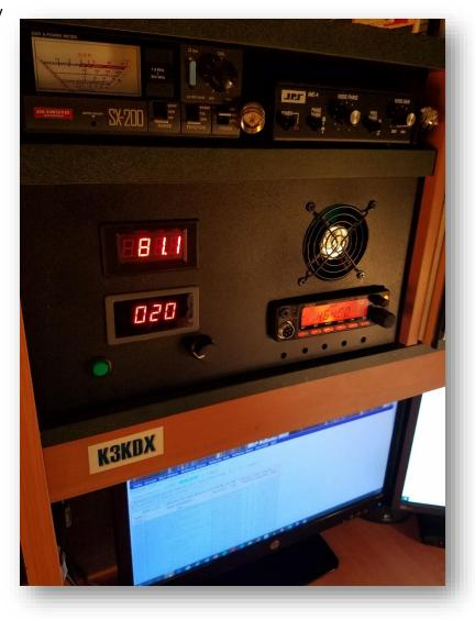
connected an alarmed temp gauge and a fan controller for the two 80mm fans that I installed.
